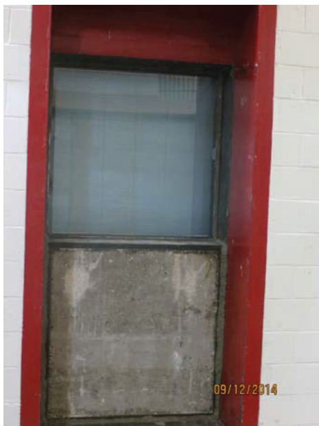
Figure 1 - Specimen mounted in the test frame.
